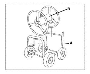
**4.** Insert reel assembly hub into crank stem and line up holes. Insert two carriage bolts (H3) from top and side of the crank hub and tighten using enclosed wrench or adjustable wrench.
